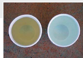
Before and after: Four Way WSC water before ozonation, left; and after, right
